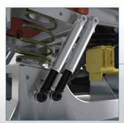
Springs and shock-absorbers reduce floor vibration. This means lower noise and increased comfort of use at the laundry.
